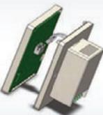
Carefully unplug the ribbon connector which is plugged in to the front half of the thermostat
