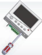
Carefully separate the front half of the thermostat from the back plate by placing a small flat head terminal driver into the slots on the bottom face of the thermostat.
